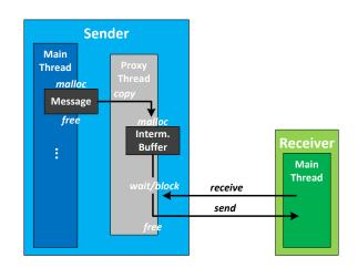
The thread receiving an asynchronous message queries for pending messages. The receiver can potentially block on the proxy thread if no message is to be transmitted.
